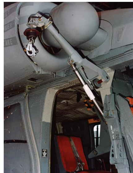
Full-time, 600 lb capacity, rescue hoist.
