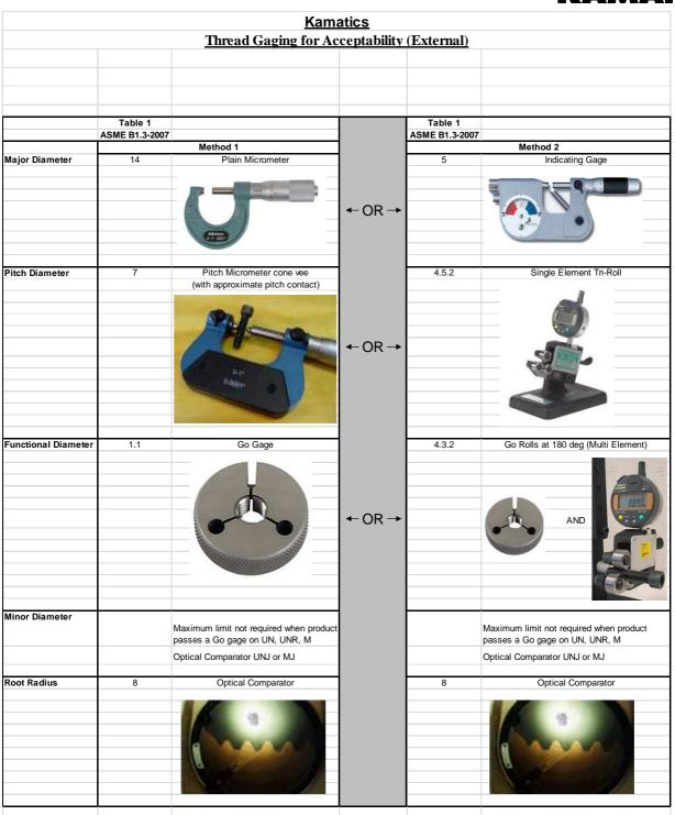
**TABLE 1 (con't)** - External Threads Inspection Methods
